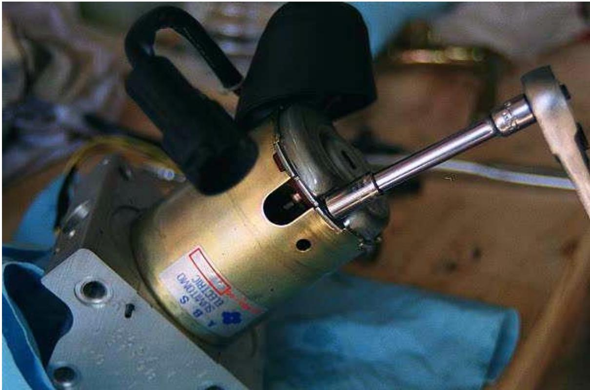
3) Remove 8mm hex nuts. Note: In the picture, I removed the plug while the HU was still in the bike. The next step is much easier to do with the HU on the bench.
